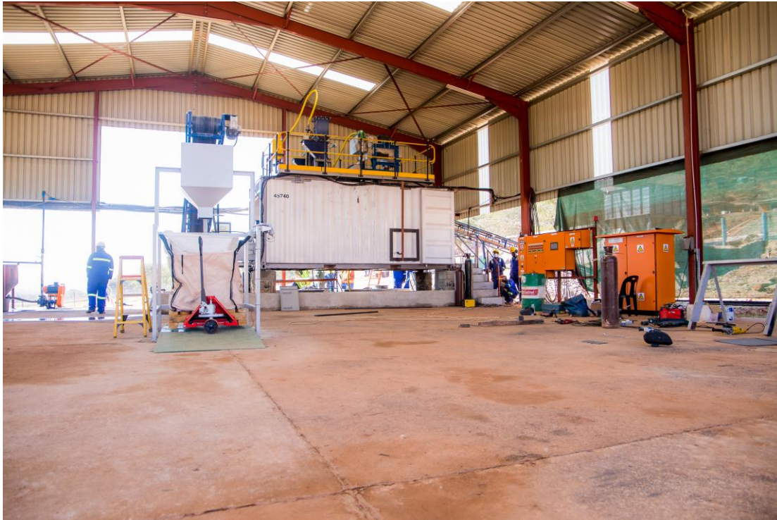
Figure 1 – Dense Media Separation (DMS) unit
